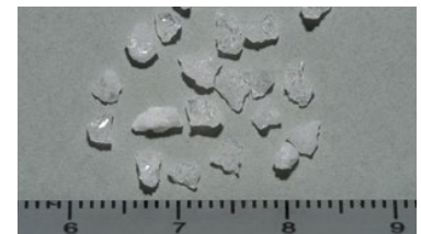
Pic. 8 Grit blasting material (sharp edged & large diameter) (available at MetaLine®)
