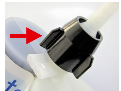
Pic. 33 Union nut - securely tighten manually
