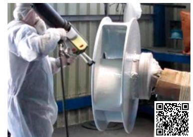
Video 21.2 Spraying technique on vertical rotating devices
