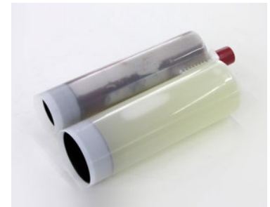
Pic. 39 Settling of color pigments (small cartridge)
