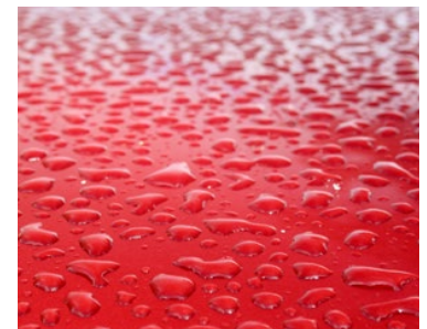
Pic. 13 Condensation of air moisture on a cold substrate (greatly enlarged)
