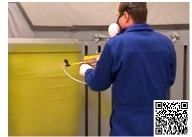
Video 21.1 Spraying technique on vertical surfaces
