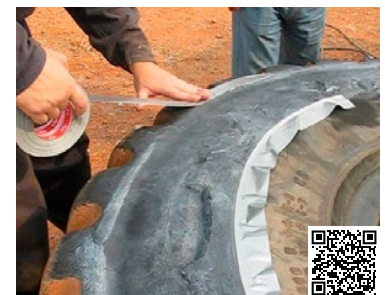
Video 7.2 Masking of edges with duct tape
