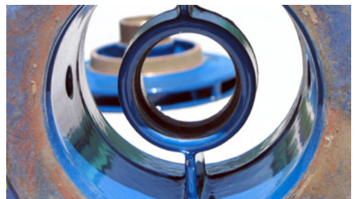
... and that's the way it should be! The MetaLine resurfacing technology is smoother than any steel casting and about 500 % more wear-resistant compared to mild steel . Repairs extending the durability of original spare parts and offering lower maintenance costs!
