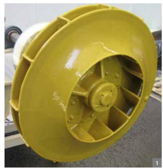
The remarkably low density of only 1,05 kg/m² per mm film thickness (0.215 lbs/ft²/40 mil) keep equipment weight low. Impact and erosion-resistant. Electrically non-conducting (must not be used in "EX"-areas). Suitable up to 70 m/s (230 ft/s) of centrifugal speed. Up to 5 dB(A) sound deadening in terms of structural borne noise.
