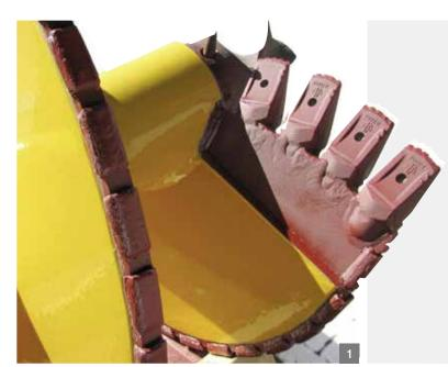
If material builds up like "glued", wear resistant, non-stick coatings are a preferred solution to get back the efficiency of earth moving equipment.
