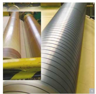
Sprayable elastomeric compouds for the repair of existing linings or complete new roller coatings. Available hardnesses 60 / 85 / 95 Shore A in a seamless quality. End-faces can be covered as well.
