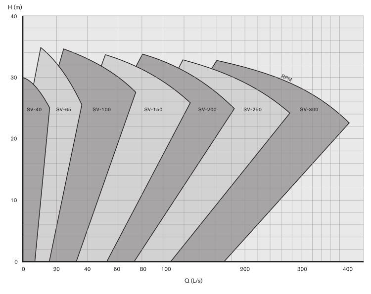
The selection chart should be used as a basic guide only. This chart indicates the range and quantity of flow available from pumps with standard impellers. It can also, however, be used to obtain a preliminary pump selection providing the user is able to estimate the quantity of slurry to be pumped and the developed head required.
