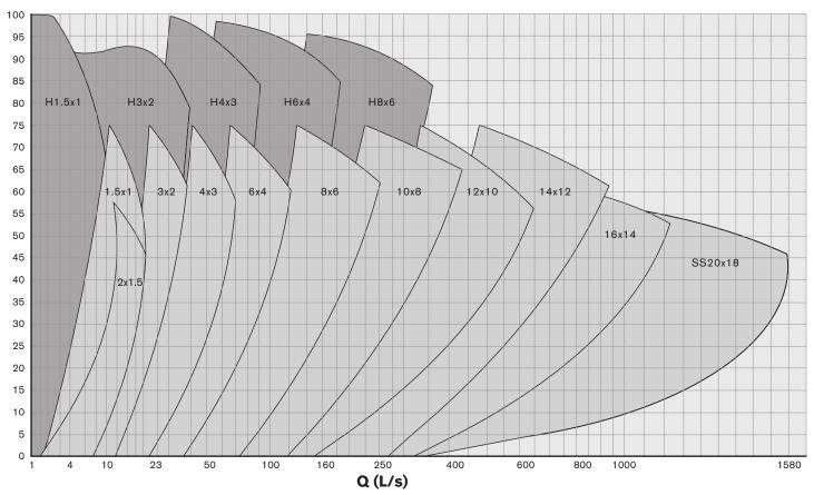
The selection chart should be used as a basic guide only. This chart indicates the range and quantity of flow available from pumps with standard impellers. It can also, however, be used to obtain a preliminary pump selection providing the user is able to estimate the quantity of slurry to be pumped and the developed head required.
