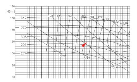
Manufacturers provide a table showing flow rates at different head pressures. As you increase the flow rate, the friction loss increases. Just follow their guidelines! However, no matter the size of your pump, there will be an efficiency limit.
