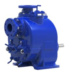
The TORO self-priming trash pumps are designed to move heavy and viscous fluids containing abrasive particles and large, soft solids. There are a wide variety of sizes and high head versions available, in cast iron, 316 stainless steel or duplex standard construction.
