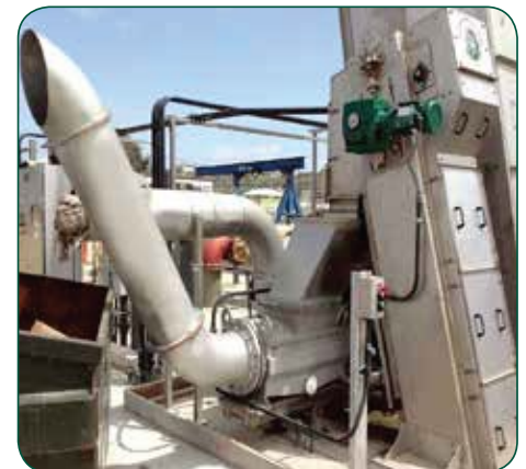
A Chain and Rake Monster Discharges into an optional Screenings Washer Monster for a cleaner, drier discharge
