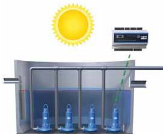
Pumping Water No Higher Than Needed Keeping start/stop levels at optimal height in order to save pumping energy
