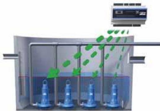
Preventing Clogging With Individual Exercise Runs Reducing the risk of clogging with individual pump running schemes
