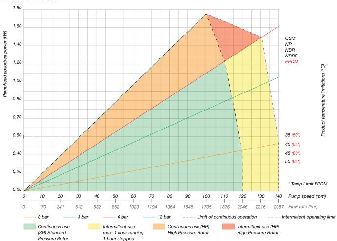
Any application below 15 Hz may require special review. Flows are typical and were measured with water at 20°C with no suction lift or discharge pressure. Actual flows will vary according to suction conditions, discharge pressure and normal component production tolerances.
