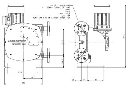
N.B. GMU AND MOTOR SHOWN: -MOTOVARIO NMRYP\_063 WITH FA OUTPUT FLANGE AND 71 FRAME B5 FLANGE MOTOR.
